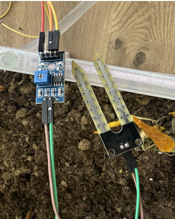
Figure 3.7. Soil moisture sensor module used during prototype testing.
