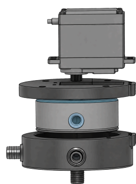
Figure 2.6. Exploded view of the rotary manifold assembly, showing the manifold body, internal rotor, top cover, and MG996R servo motor.
