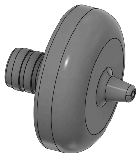
Figure 2.1. Isometric view of the final single outlet emitter model developed in Autodesk Fusion 360.
