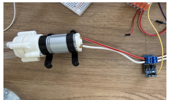
Figure 3.5. R385 DC pump connected to the MOSFET switching module during prototype wiring and functional testing.
