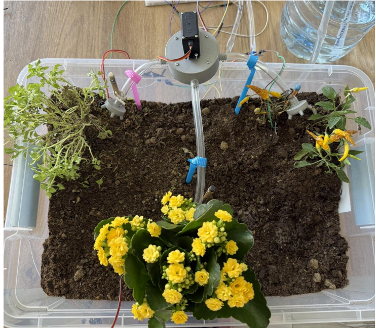
Figure 4.3. Integrated three zone prototype used for moisture guided servo selection, showing the Yellow Pepper, Basil, and Kalanchoe irrigation zones connected to the servo-controlled rotary manifold.
