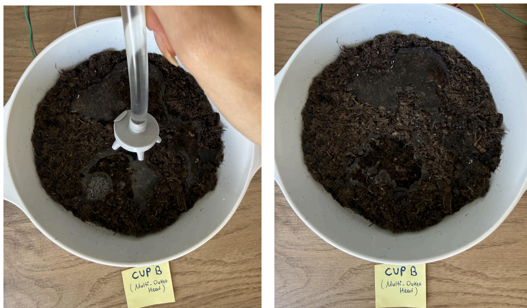
Figure 5.5. Multi outlet emitter wetting pattern during the equal volume test.
