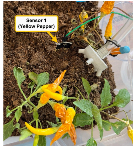
Figure 3.9. Sensor 1 installed in the Yellow Pepper zone, showing the capacitive soil moisture sensor positioned in the soil adjacent to the irrigation emitter.
